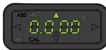
Figure 5. Device display in Alternate zero mode
